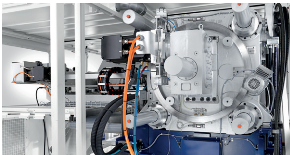
The electric clamping unit works precisely and is gentle to the mold
