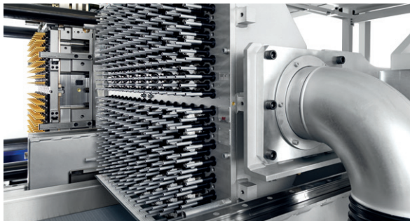
Fully integrated post-mold cooling unit with internal and external preform cooling
